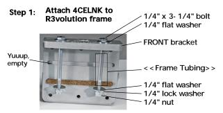
Position so the cork pad is tight against the rail, and tighten the bolts so it all stays in place. Don't overtighten, though.
